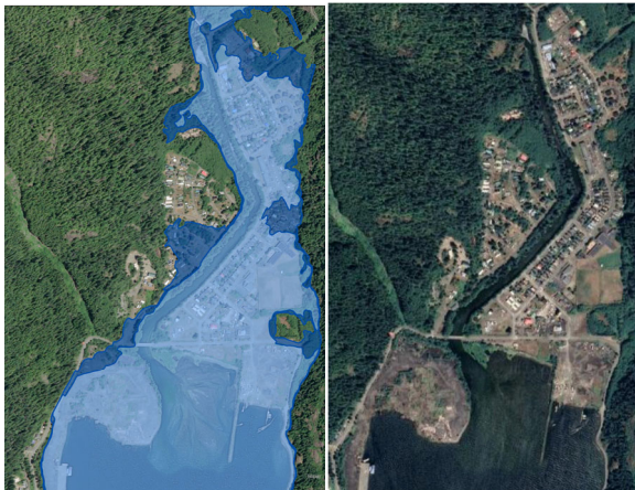
FIGURE 3. (Left) Inundation extent map for a Cascadia tsunami in Tahsis, BC, produced by the Northwest Hydraulic Consultant Ltd. in collaboration with ONC. (Right) Satellite image of Tahsis, BC, showing existing shoreline without inundation extent.
