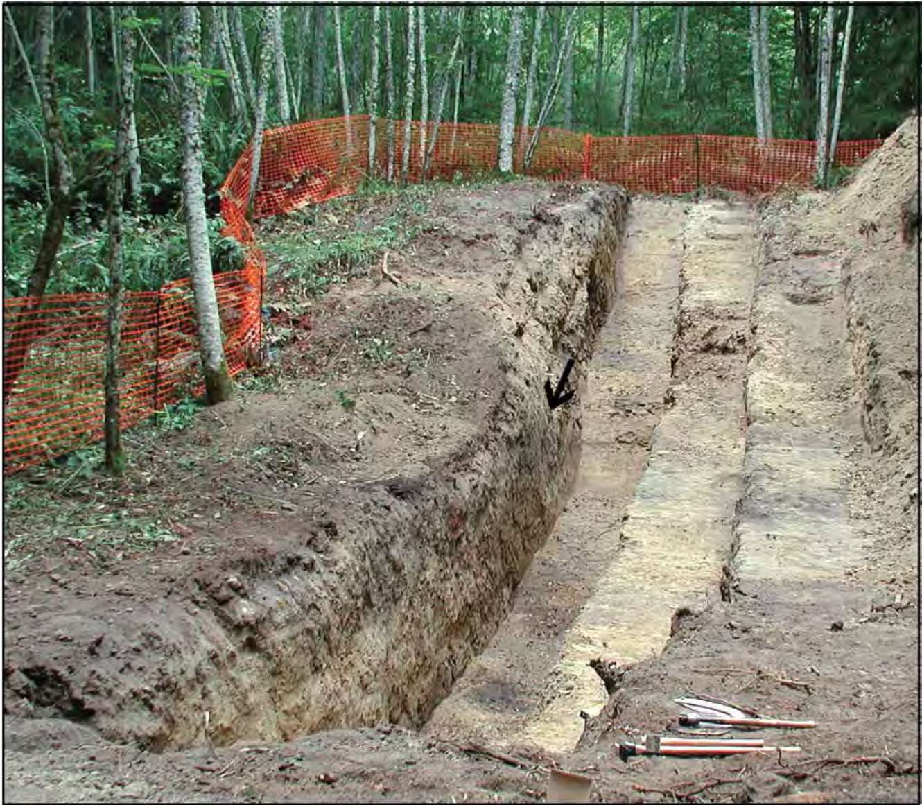
Figure 9. Nettle Grove trench on the Waterman Point fault looking northwest. Fault is highlighted by color contrast at black arrow in center of photo. From U. S. Geological Survey Miscellaneous Field Studies Map MF-2423.
