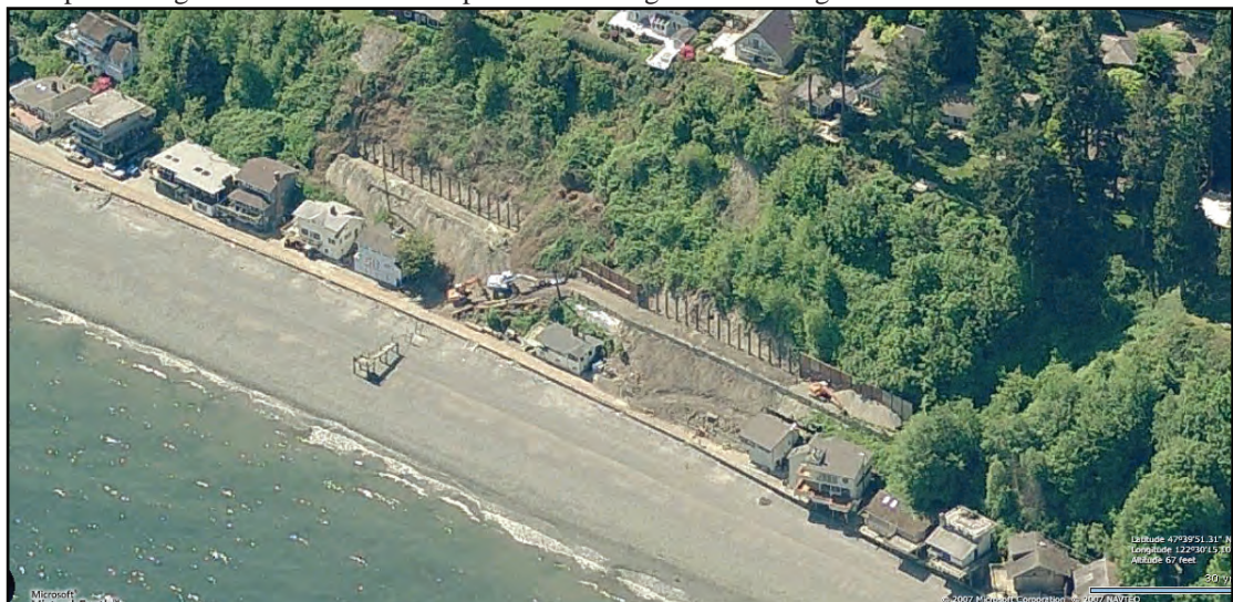
Below: Oblique aerial view of the same area after the debris was removed and remediation of the slope has begun. Note the newer slope failure through the retaining wall under construction.
