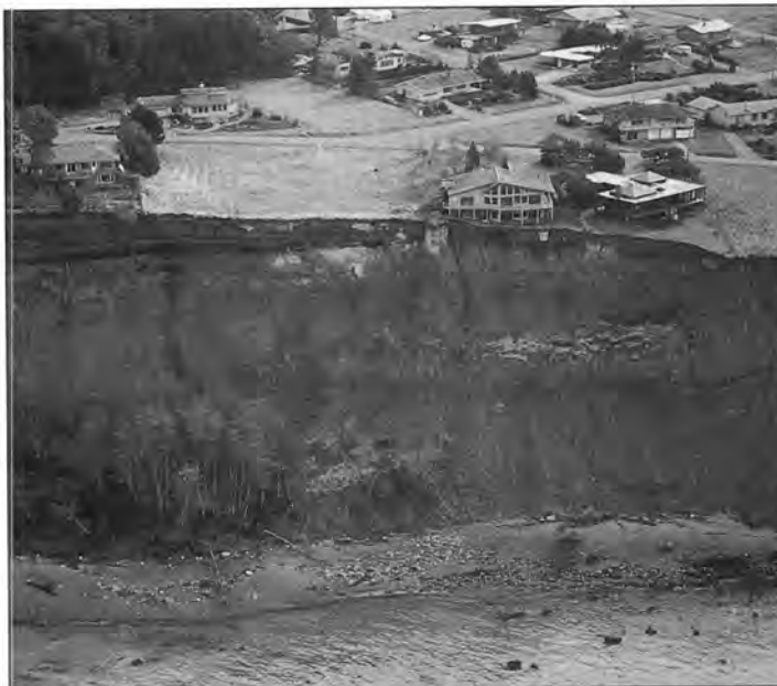
Figures 19A & B. Continuing slide activity has made this home near Cape George in Jefferson County uninhabitable. At this site, the perching layer is a small area of ancient lakebed silt that lies beneath the house at about mid-bluff level, now covered with grass dropped from the back lawn. This part of the bluff remains green year round. Note the old slide mass at beach level (lower left), now covered by alder trees that are all of approximately the same age (here, perhaps 25 years old). Also note the arcuate line of boulders seaward of these trees. Such a pattern of boulders, which are commonly accompanied by steeply tilted silt and clay beds, can indicate an old slide surface at or below beach level. B. (right) This closeup shows recent slide debris on the bench, as well as the exposed septic tank (the white rectangle below the right side of the house and drainfield pipe in A); the tank has since fallen to the beach. Poorly located septic systems often contribute to slope instability. The dark strata at the upper part of the bluff are gravels and are not saturated here. It is possible that drainfield effluent percolated downward and bluffward to destabilize this slope or that deeper ground water caused the problem at this location. Wave erosion has likely been a contributor at this site as well. Trying to maximize a view by building close to the bluff line can be a costly and potentially hazardous mistake.
