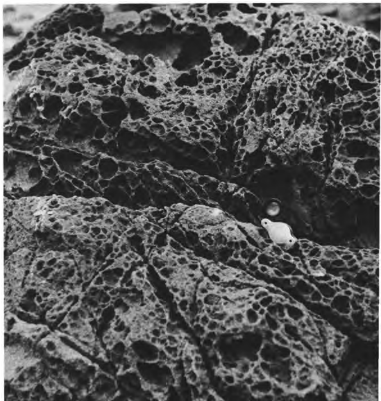
FRETTE D SANDSTONE SURFACE. Sandstone surfaces that are dampened by sea spray and dried periodically can become delicately weathered. Slight variations in the resistance to erosion within the sandstone results in a honey-comblike surface structure (fig. 64).
