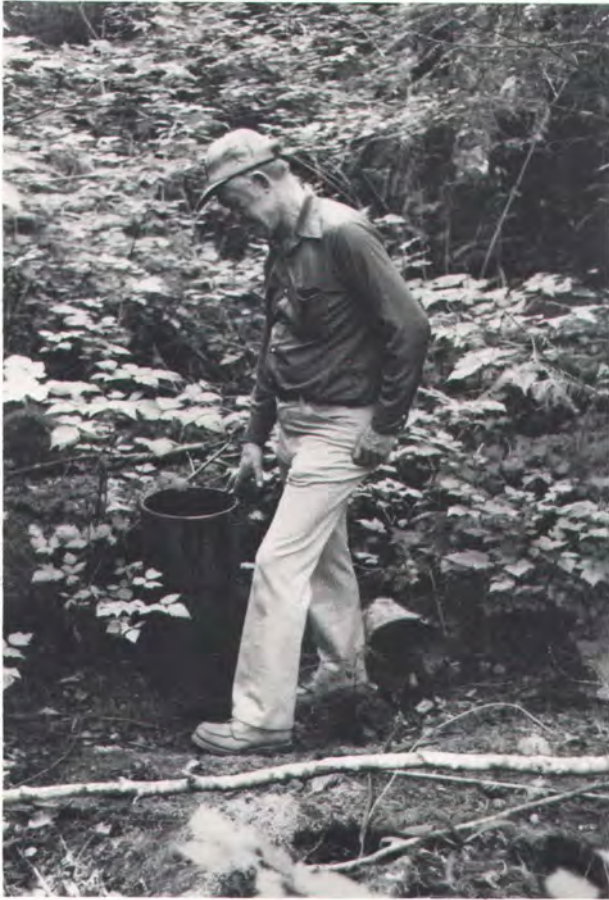
OIL WELL REMAINS from drilling operations of the 1930's near Hoh Head. Gas still bubbles from, and oil accumulates in, this casing (fig. 22).
