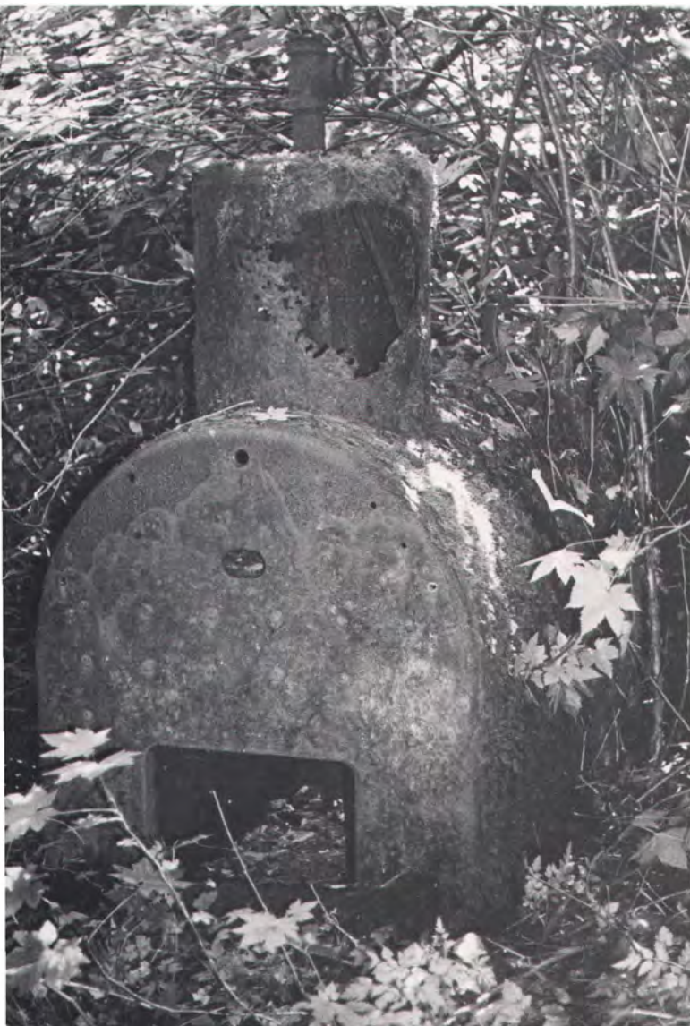
THIS STEAM BOILER is among the remains of equipment used to drill an exploratory oil well during the turn of the century near Third Beach (fig. 59).
