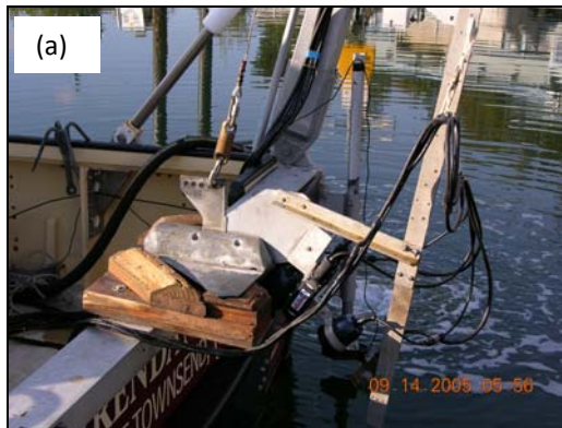
Figure 2-6. The R/V Brendan D II is equipped with a weighted towfish that contains an underwater video camera mounted in a ‘downward looking’ orientation, dual lasers for scaling reference, and underwater lights for night work (a). The towfish is deployed directly beneath the DGPS antenna attached to the A-frame cargo boom, ensuring accurate geographic location of the camera (b).
