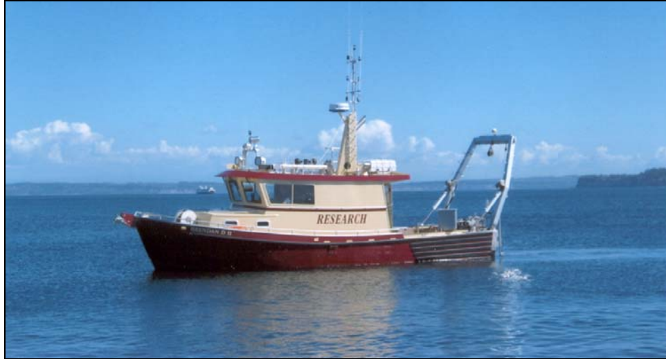
Figure 2-5. The R/V Brendan D II owned and operated by the Marine Resources Consultants. Eelgrass ( Z. marina ) presence and depth distribution data was collected at the Maury Island AQR sites and the northern portion of the Fidalgo Bay AQR site ( flats15N-Fidalgo Bay North ) from the R/V Brendan D II using underwater videography and depth sounding instrumentation. A small research skiff and BioSonics echosounder were used to sample eelgrass at the southern portion of the Fidalgo Bay AQR site ( flats15S-Fidalgo Bay South ).
