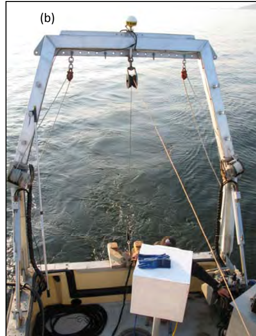
Figure 2-4. The R/V Brendan D II is equipped with a weighted towfish that contains an underwater video camera mounted in a ‘downward looking’ orientation, dual lasers for scaling reference, and underwater lights for night work (a). The towfish is deployed directly beneath the DGPS antenna attached to the A-frame cargo boom, ensuring accurate geographic location of the camera (b).
