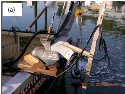
Figure 2-4. The R/V Brendan D II is equipped with a weighted towfish that contains an underwater video camera mounted in a ‘downward looking’ orientation, dual lasers for scaling reference, and underwater lights for night work (a). The towfish is deployed directly beneath the DGPS antenna attached to the A-frame cargo boom, ensuring accurate geographic location of the camera (b).
