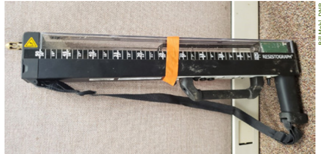
Photo 6. Resistograph. The bit is inserted into the wood to measure resistance. Soft, rotted wood has a resistance near zero.
