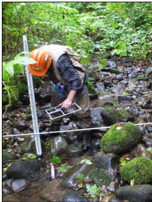
Figure 9. Sampling channel course substrate using a stadia rod and gravelometer.
