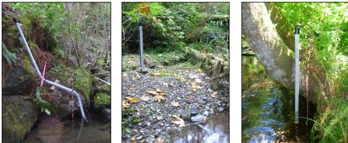
Figure 18. Stream gage designs: a) over-bank housing in basin 694; b) in-bank housing in basin 145; c) vertical housing in basin 433
