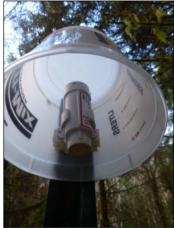
Figure 21. Microclimate transect (a) and microclimate data logger and shade housing (b).
