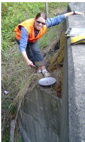
The gravimeter goes here! Risky benchmark gravity reading: a bridge abutment outside the rail. Oh the lengths I go for good data.
