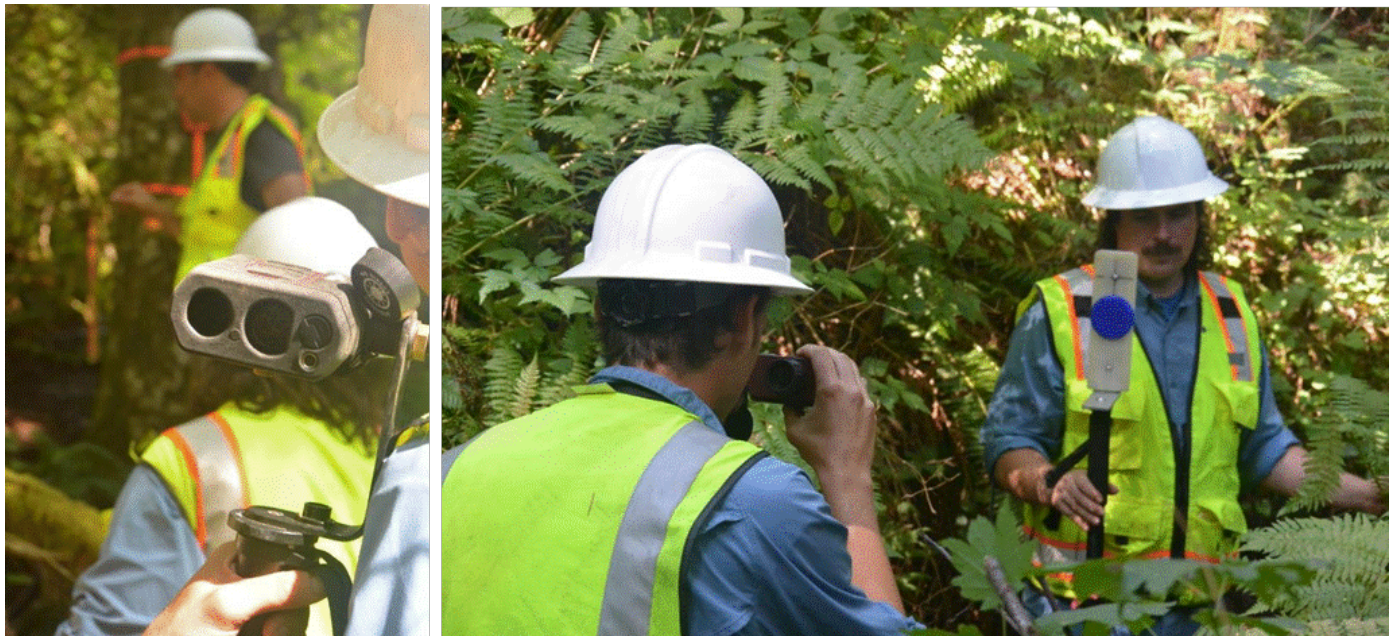
Figure 2. Photos of crew using laser range finder and target mounted on monopods to survey longitudinal profile and stream characteristics for PHB Pilot Study.
