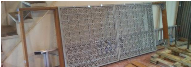
A dock before installation showing one grating design being tested; Eco Series Steel Deck 60% multidirectional open space.
