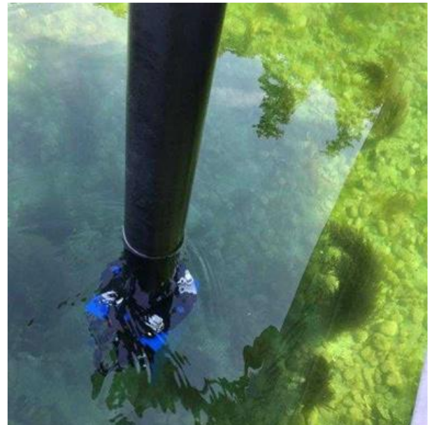
AAMT's multibeam sonar system is configured to collect data in the shallow intertidal. Shown here is the sonar operating in 1 to 2m of water.
